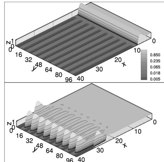
FIG. 1. Contour plot of the flow over a striped substrate. (a) Initial configuration (the straight contact line is at  $x=7$ ). (b) Well-developed fingers propagating between the channels. The width of the channels is  $w=3.5$ , the distance between their centers is  $d=10$ , and they are imposed at  $x_c=10$ . Note that  $y=48$  is a symmetry line;  $b_0=0.01$ .
