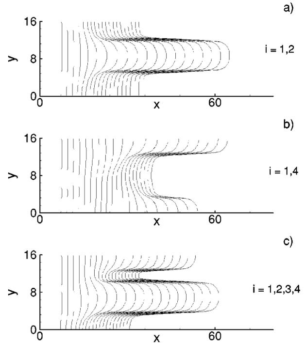
FIG. 14. (a) Snapshots of the contact line at  $\delta t=2$  intervals where initially more than one mode is present ( $\lambda_{0,i}=2L_y/i$ ). (a)  $i=1,2$ , (b)  $i=1,4$ , (c)  $i=1,2,3,4$ . All other parameters are as in Fig. 4.
