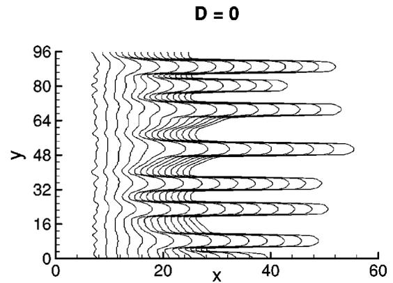
FIG. 15. Snapshots of the contact line in  $\delta t=2$  intervals for the flow down a vertical plane ( $L_y=96$ ,  $N=50$ ,  $b=0.01$ ,  $\Delta x=0.2$ ,  $\Delta y=0.5$ ).
