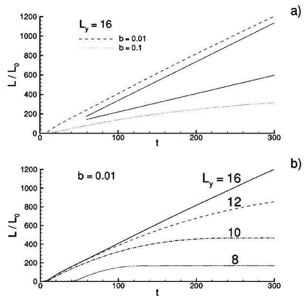
FIG. 11. (a) Long time evolution of the length of the emerging patterns for  $D = 0$  and different  $b$ 's. The solid lines emphasize the linear growth for  $b = 0.01$ , and the deviation from linear growth for  $b = 0.1$ . (b) Length of the emerging patterns for  $D = 0$  and different  $L_y$ 's. All other parameters are as in Fig. 4, except the box sizes in the  $x$  direction, which are  $L_x = 200$ .
