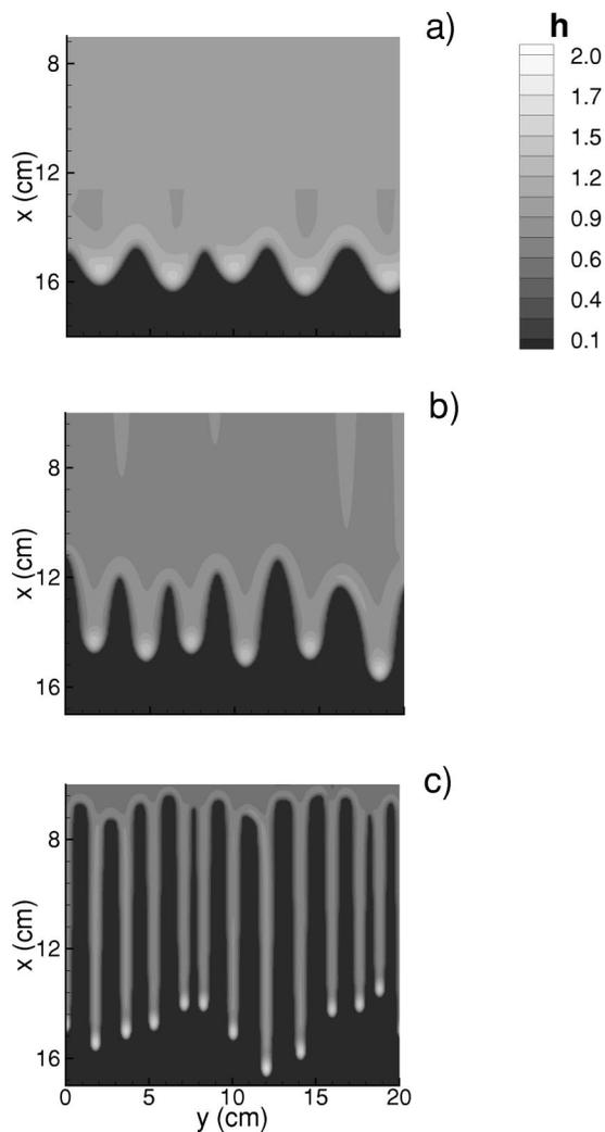
FIG. 21. Contour plots of fluid profiles for (a)  $D=0$ ; (b)  $D=0.67$ , and (c)  $D=1.34$ , plotted when the fluid traveled the same distance downslope. All other parameters are as in Fig. 15. Note that the  $x$  and  $y$  scales are in cm, and fluid thickness,  $h$ , is in mm.
