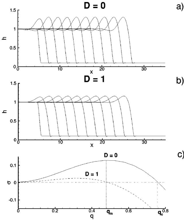
FIG. 2. Profiles of a film flowing down a vertical plane (a), and down an inclined plane (b). The time interval between profiles is  $\delta t=2$ , the grid size is  $\Delta x=0.05$ , and  $b=0.1$ . (c) Growth rate  $\sigma$  following from LSA vs wave number  $q=2\pi/\lambda$  for  $D=0$  and  $D=1$ . The wavelength of maximum growth is  $\lambda_m=2\pi/q_m$ , and the critical wavelength is  $\lambda_c=2\pi/q_c$ .
