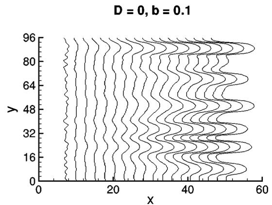
FIG. 18. Snapshots of the contact line in  $\delta t=2$  intervals for the flow down a vertical plane. Here  $b=0.1$ ; all other parameters are as in Fig. 15.
