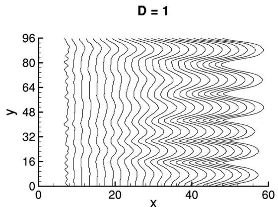
FIG. 19. Snapshots of the contact line for the flow down an inclined plane  $D=1$  in  $\delta t=5$  intervals. All other parameters are as in Fig. 15.
