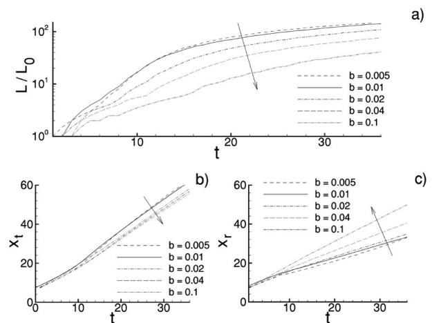
FIG. 6. Influence of the precursor thickness  $b$  on (a) length of the finger, (b) position of the tip, and (c) position of the root. Other parameters are as in Fig. 4. The arrows show the direction in which  $b$  is increased.
