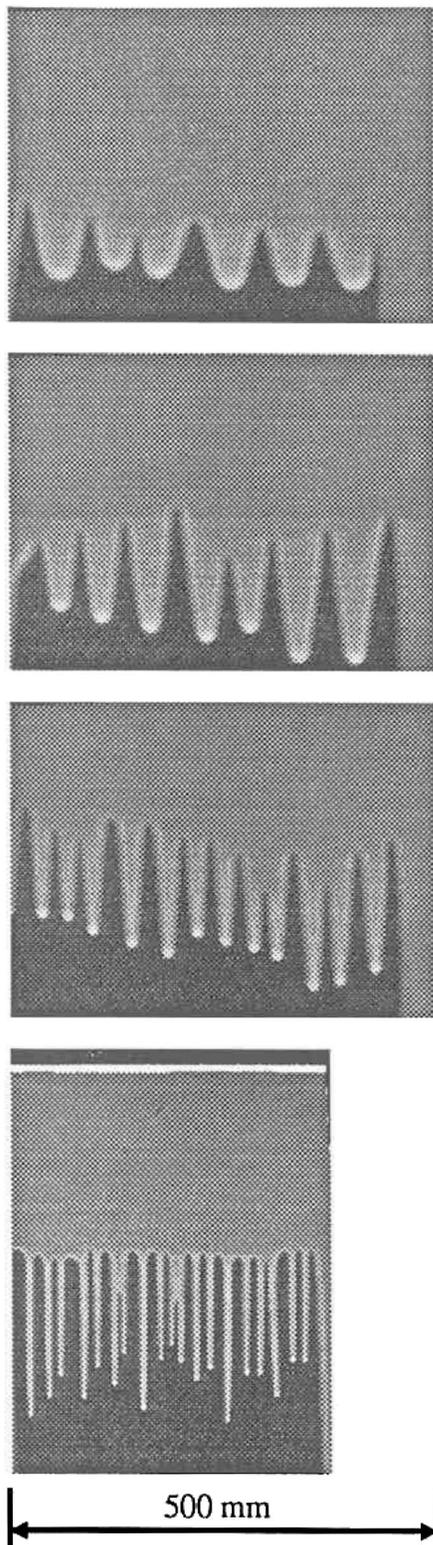
FIG. 1. Patterns formed in constant flux experiment by Johnson (Ref. 7). The fluid is glycerine–water mixture (more details about this experimental setup are given in Sec. V B), and the inclination angle is (from top to bottom)  $\alpha=7.2^\circ$ ,  $13.9^\circ$ ,  $27.9^\circ$ , and  $90.0^\circ$ . The profiles are shown after the fluid traveled the same distance down an incline. (Reproduced with permission of the author.)
