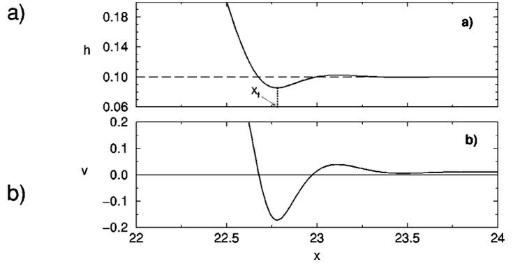
FIG. 3. Fluid thickness and velocity profile of the film near the apparent contact line for  $D=1$  and  $b=0.1$ .
