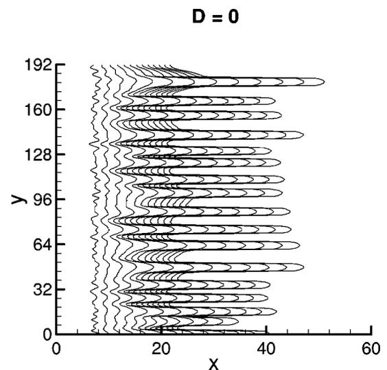
FIG. 16. Snapshots of the contact line in  $\delta t=2$  intervals for the flow down a vertical plane ( $L_y=192$ ,  $N=100$ ). All other parameters are as in Fig. 15.
