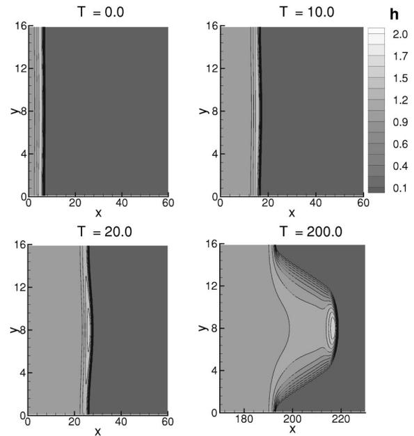
FIG. 8. Contour plot of the flow down an inclined plane ( $D=1$ ). All other parameters are as in Fig. 4.
