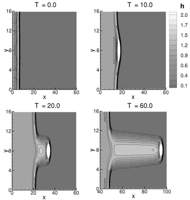
FIG. 4. Contour plot of the flow down a vertical plane perturbed by a single mode characterized by  $A_0 = 0.1$  and  $\lambda_0 = 16$ . The precursor film thickness is  $b = 0.01$ , and the grid spacing is  $\Delta x = 0.2$ ,  $\Delta y = 0.25$ .
