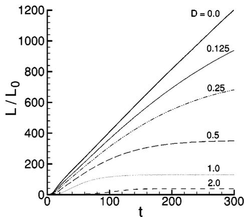
FIG. 10. Length of the emerging patterns for different  $D$ 's. All other parameters are as in Fig. 4, except the box sizes in the  $x$  direction, which are  $L_x = 200$ .
